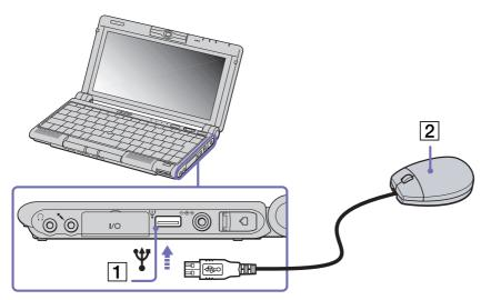
A You can connect the optional Sony USB mouse (PCGA-UMS1 series). As the driver for this mouse is preinstalled on your computer, you can use the mouse by just connecting it.
